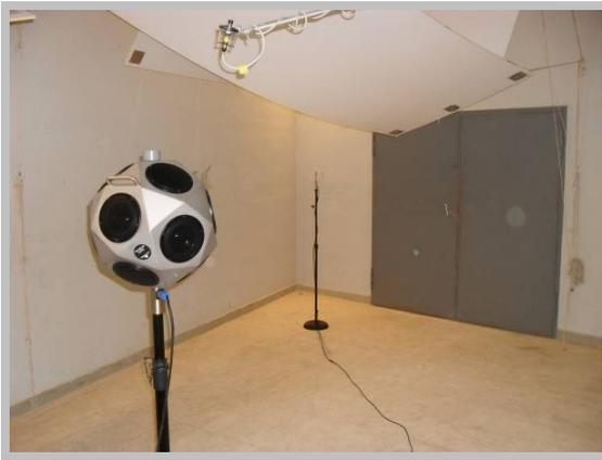
**Figure 1.** Diffuse-field measurement in reverberation room
