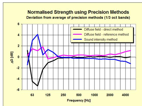
**Figure 7.** Normalised G obtained from precision calibration methods, presented in 1/3 octave bands
