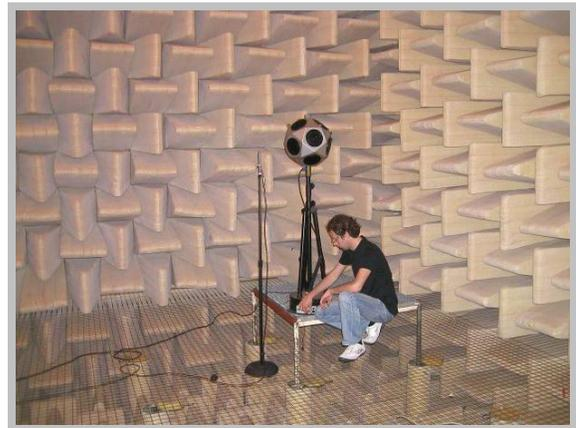
**Figure 3.** Free-field measurement in anechoic room
