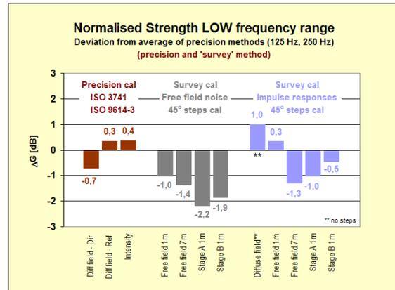
**Figure 11.** Normalised low frequency (avg 125 - 250 Hz) wide band value of G for all calibration methods
