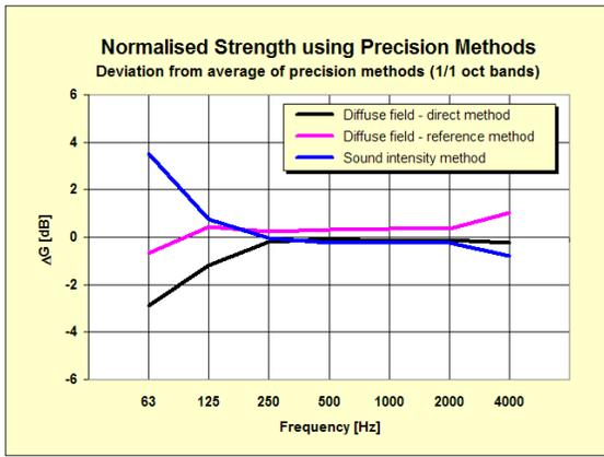
**Figure 8.** Normalised G obtained from precision calibration methods, presented in full octave bands
