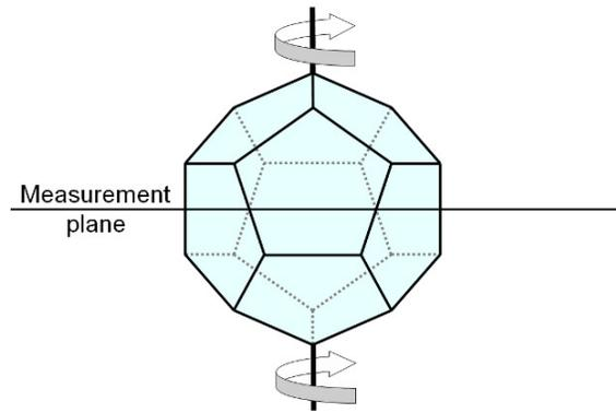
**Figure 2b.** Side view of vertical rotation axis and horizontal measurement plane during free-field and near-field measurements
