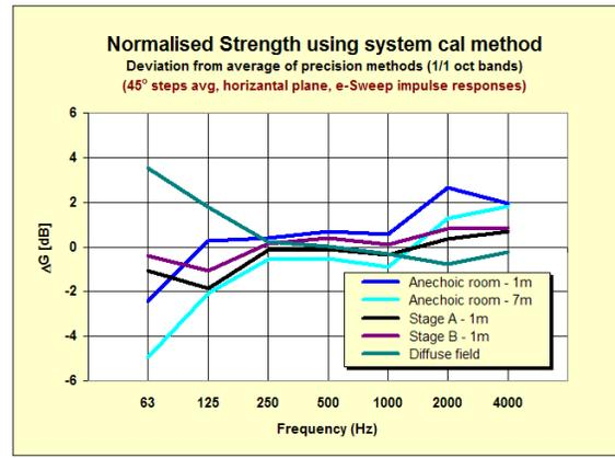
**Figure 10.** Normalised G obtained from impulse response measurement using e-sweeps and deconvolution
