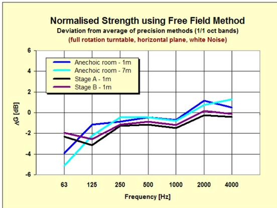
**Figure 9.** Normalised G obtained from free-field calibration methods using white noise
