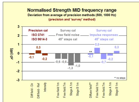
**Figure 12.** Normalised mid frequency (avg 500 - 1000 Hz) wide band value (= single number value according to ISO 3382-1) of G for all calibration methods
