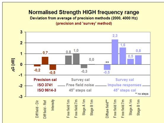
**Figure 13.** Normalised high frequency (avg 2 kHz - 4 kHz) wide band value of G for all calibration methods
