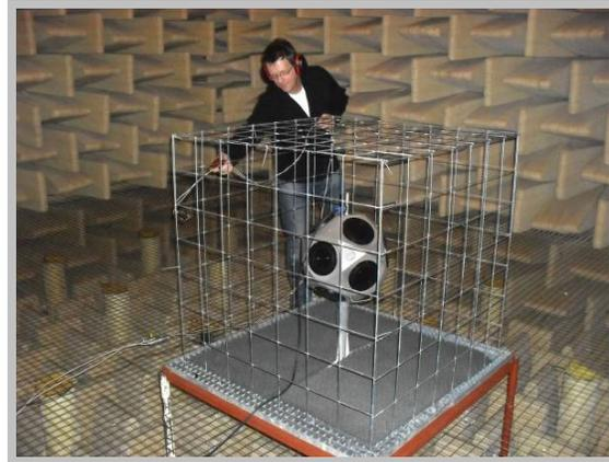
**Figure 6.** Sound Intensity measurement in anechoic room
