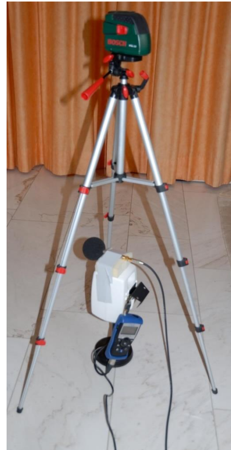
The IR light line on the walls allow you to position the bottom of the ball before dropping it.
